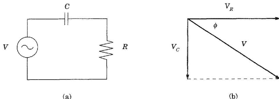
Figure 37.1  $RC$  circuit and the phasor diagram for the voltage across each element.
