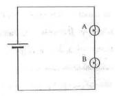
Now add another identical bulb in series as shown below and observe the bulb brightness.
